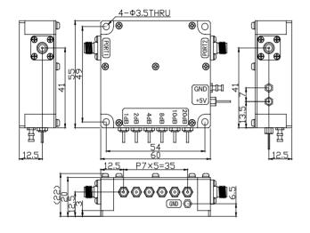
Broadband Frequency :0.01 ~ 4000MHz Attenuation : 1dB Step/6Bit/45dB
