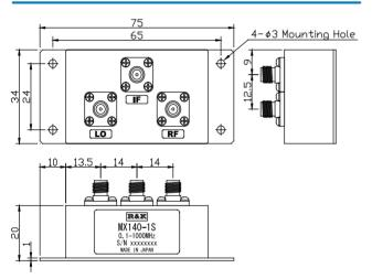
LO&RF Frequency  $: 0.1 \sim 1000 MHz$ IF Frequency Lo Drive Level :DC ~ 1000MHz : +10dBm
