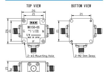
■ L0&RF Frequency■ IF Frequency■ Lo Drive Level :01 ~ 1000MHz :DC ~ 1000MHz : +15dBm
