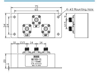
LO&RF Frequency  $: 0.1 \sim 1000 MHz$ IF Frequency Lo Drive Level :DC ~ 1000MHz : +20dBm
