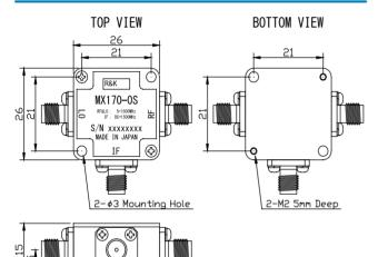
■ LO&RF Frequency ~ 1500MHz :5 ■ IF Frequency■ Lo Drive Level :DC ~ 1500MHz
