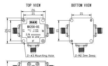
■ L0&RF Frequency■ IF Frequency■ Lo Drive Level :5 ~ 1500MHz :DC ~ 1500MHz  $\pm 20 dBm$
