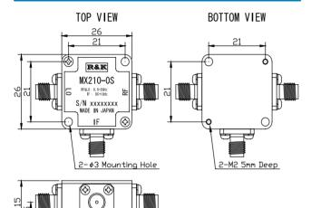
■ LO&RF Frequency■ IF Frequency■ Lo Drive Level :500 ~ 2000MHz : DC 1000MHz
