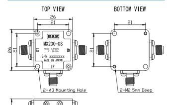
■ LO&RF Frequency■ IF Frequency■ Lo Drive Level :500 **~** 2000MHz :DC ~ 1000MHz : +15dBm
