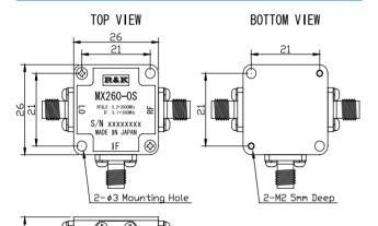
■ L0&RF Frequency■ IF Frequency■ Lo Drive Level :0.2 **~** 3000MHz :0.1 ~ 1000MHz  $\pm 15dBm$
