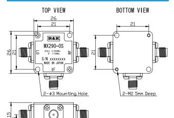
■ L0&RF Frequency■ IF Frequency■ Lo Drive Level :5 **~** 2400MHz ~ 700MHz :1
