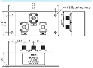
LO&RF Frequency IF Frequency Lo Drive Level :5 **~** 2400MHz :1 ~ 700MHz : +10dBm
